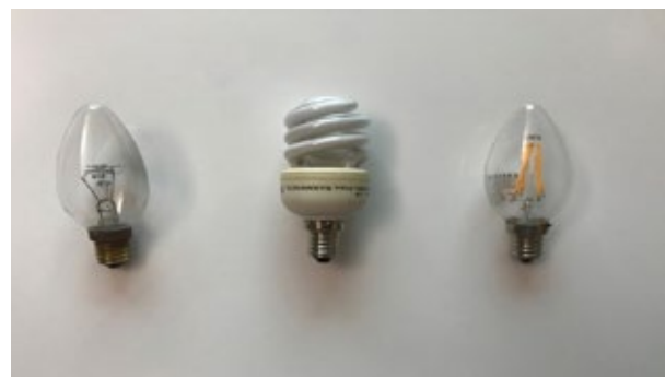
Gradual change of light bulbs for residential use: Incandescent to CFL to LED
