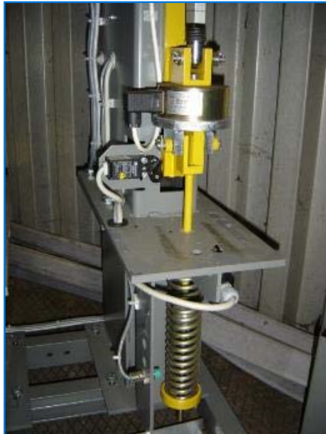
Brake shoe closed Motor with solenoid in lower end position
