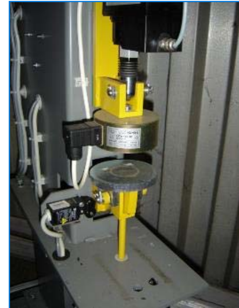
Rope brake actuated (tripped by CPD)
