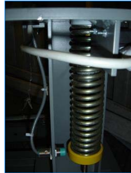
Spring tensioned, Proximity switch actuated
